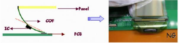
12.6 Use both thumbs to insert COF into the connector when assembling the panel. See the photo on the far right below for correct insertion of the film into the connector (one-handed insertion exerts uneven force on the film and could cause its breakage, photo on the left)
